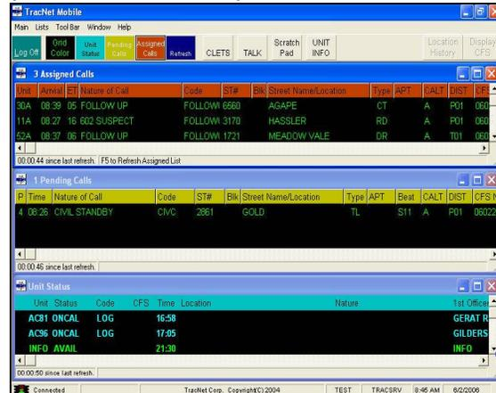
to use features of the other CAD products. The "Day/Night" feature adjusts the screen colors for bright sunlight or subtle background colors for nighttime use. Large on screen buttons are designed make touch screen use easy for officers in the field. A chat feature allows officers to communicate with each other using their mobile computers. Address history is available for all officers without dispatcher intervention.
